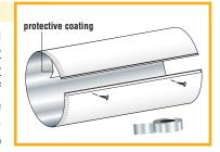
both sides of seal to ensure a good bond. Secure the tube using the provided tek screws (I) - two screws per tube. Then place foil tape (F) over the entire seam to strengthen seal.
