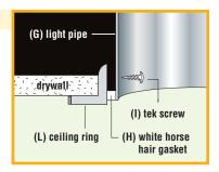
with tin snips. Secure bottom of light pipe to ceiling ring with two tek screws (I). NOTE: Use caution, light pipe is extremely sharp.
