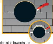
also need to be removed on the high side towards the ridge to allow the flashing to slide over hole (see inset).
