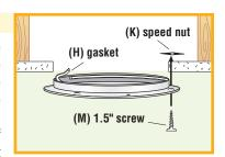
ensures a dust free fit between the light pipe and the ceiling ring. Secure the ceiling ring to ceiling by inserting a 1 1/2" Phillips flathead screw **(M)** into one of the three pre-drilled dimpled holes and screwing it up through the drywall into speed nut **(K)** provided. Repeat this process for the other two screws.
