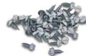
Made of zinc plated steel with painted heads. Needle point with twin lead thread. Slotted head with ¼-inch indented hex washer. All sizes stocked in white. Other colors available by special order. Larger tub quantities available upon request.
