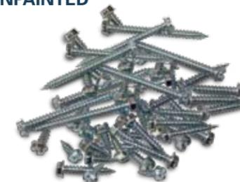
Made of zinc plated steel. Needle point with twin lead thread. Slotted head with ¼-inch indented hex. Larger tub quantities available upon request.
