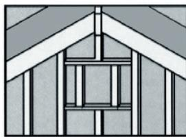
In most cases, the rough opening can be cut directly into the sheathing. However, if a non structural sheathing is used, such as an insulating foamboard, it is recommended that the opening be framed in.
