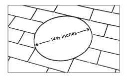
**4. CUTTING THE HOLE IN THE ROOF:** Using a sabre saw, cut and remove all roof shingles (and deck) inside the 14 1/2"-diameter circle. Next, cut an extra 1" off the top half of the hole (shingles only) to allow room for placing and positioning the flange. Do not cut through any rafters. Cutting a rafter may cause your roof to sag.
