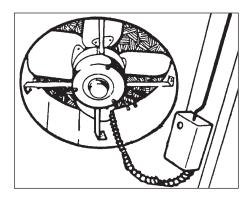
7. WIRING THE THERMOSTAT: Wire the thermostat as shown below. Attach your ground wire to the thermostat box.
