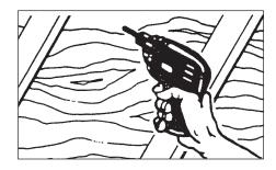
**3. CUTTING THE HOLE:** Draw a circle 14 1/2" in diameter using the guidehole as the center. A template is provided on the back of the carton for drawing the circle.
