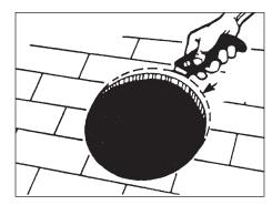
**5. SECURING THE BASE:** Make sure the base flange parallels the ridgeline of the roof. The embossed arrow
