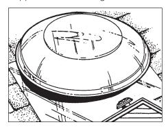
Center unit over the hole (as shown above). Attach flange securely to roof using roofing nails around the perimeter of the unit (underneath shingles at the top). A nonhardening caulk can be used as a seal between the flange and shingles.
