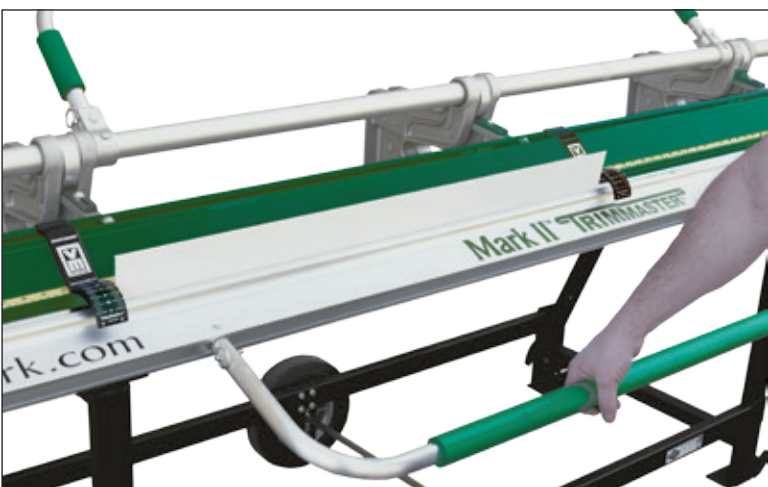
Gauge radius is positioned closer to the bend for easier sighting on material
