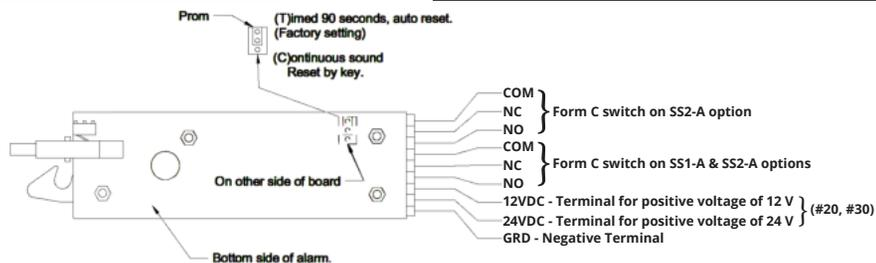
Wiring for SS1-A and SS2-A, 12 or 24 VDC External Power
