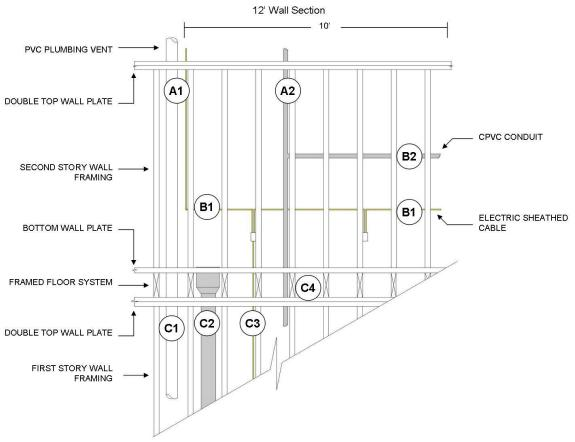
A1: **PVC** plumbing vent and electric sheathed cable at vertical penetration at ceiling level, trough double top must plate, be sealed with fire block foam
